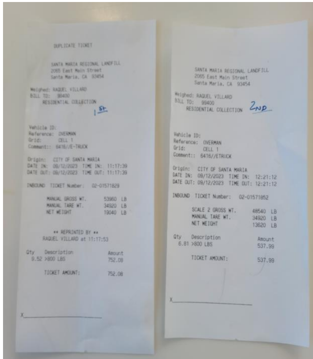
Receipt of weigh-in and out at landfill, depicting truck's physical payload capabilities.
